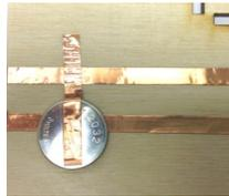
Now your battery is touching both sides of the road. One side is the *positive trace* and one side is the *negative trace*. You can use a binder clip or a piece of transparent tape to keep the switch closed if you do not wish to hold it down.
