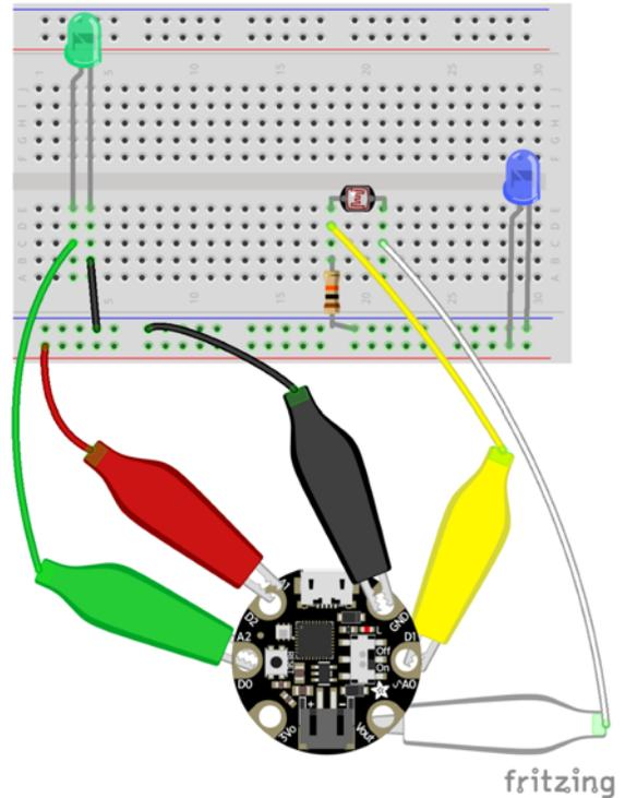
**Be careful not to connect the LED to the 3Vo pin. It may output too much voltage and burn out the LED.**
