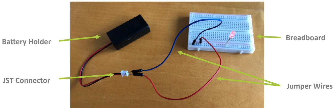
Connect a blue LED by pushing the anode (longer leg) into any tie on the red (+) strip and the other leg (the cathode) into the blue (-) strip. If all your connections are tight, you should see the LED light.
