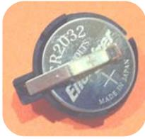
Connect the battery to the breadboard by connecting the prong near the tab on the battery to the red strip (positive) and the other to the blue strip (negative or ground).
