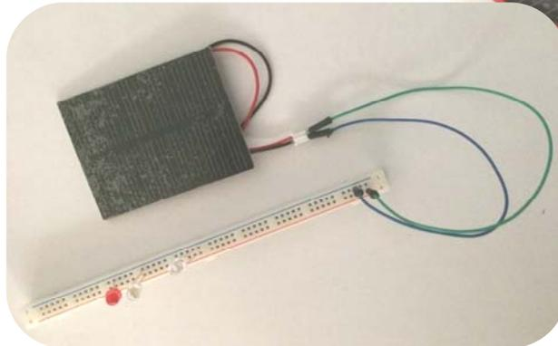
**Use the solar panel with the breadboard.** Push one end of each the jumper wires into the connector on the solar panel.
