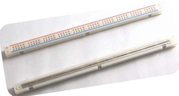
many sizes. This breadboard has two parallel strips of conducting metal along the length of each side. Each strip has fifty connected holes, called tie points, but the two sides do not touch each other.
