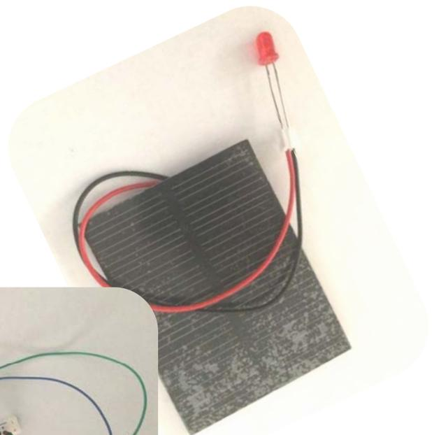
Photovoltaic (PV) cells, or solar cells produce electricity directly from light. PV powered calculators have been common for many years, and PV cells have become especially useful for providing electricity in places that are not near conventional sources. Where do you see solar cells?
