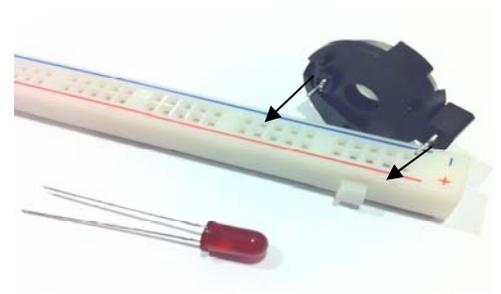
Connect an LED by pushing the anode (longer leg) into a tie on the red (+) strip and the other leg (the cathode) into the blue (-) strip. If all your connections are tight, you should see the LED light.
