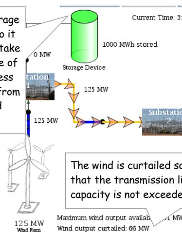
The wind is curtailed so that the transmission line capacity is not exceeded.
