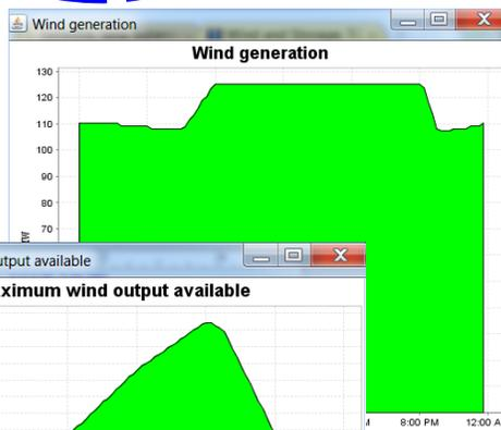
The wind generation plot shows generation of 125 MW between approximately 8:00 AM and 8:00 PM, but the maximum wind output available shows more wind power available during these times. The utility needs to consider whether to increase the transmission capacity to take advantage of all the available wind power.
