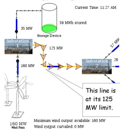
However, the wind is not yet curtailed because the storage is taking the excess energy.
