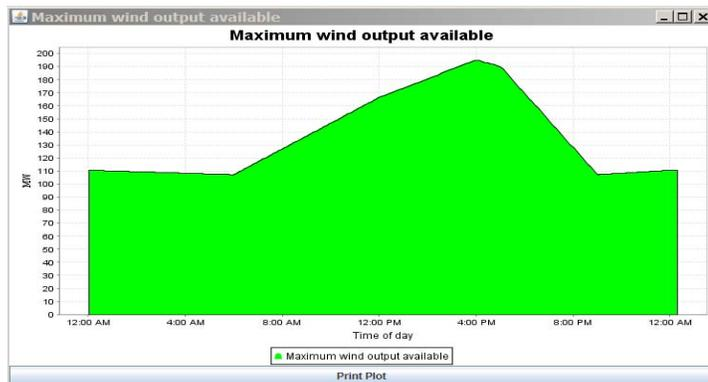
The turbines in the wind farm could generate this maximum power if no wind is curtailed.
