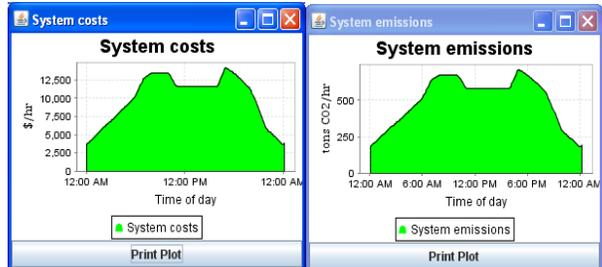
When the peak demand is 750 MW and the wind farm is not connected, only the coal generator is producing electricity.
