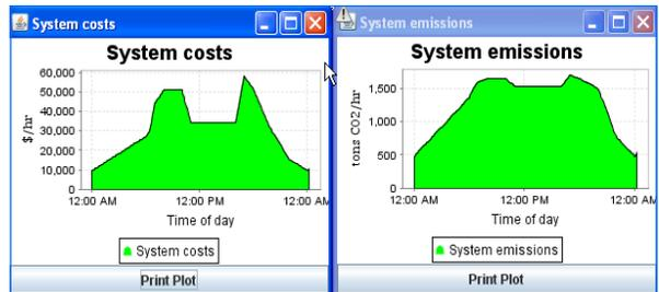
When the peak demand is 2000 MW and the wind farm is not connected, the coal generator produces the first 1500 MW of electricity and the natural gas is producing the rest.
