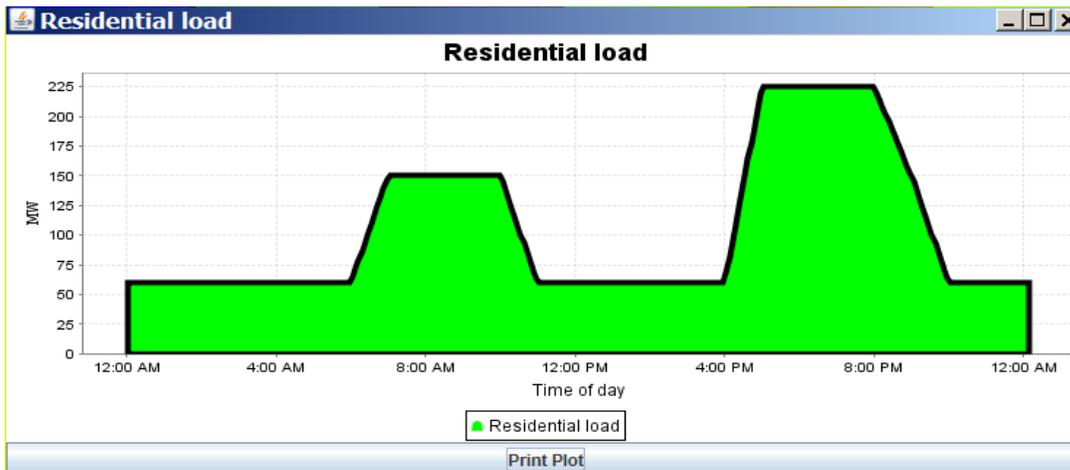
Power utilities encourage residential customers to consider moving some of their electricity use to the times of day when typical demand is lower. Some utilities are installing electricity meters that can record energy use hourly. These allow the utility to offer plans that charge lower prices when demand is low and higher prices at times when the demand is higher. There are a variety of these plans offered by various utilities.
