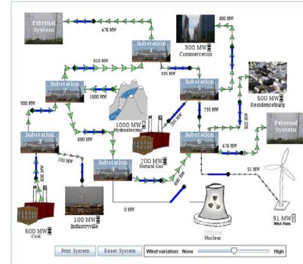
The **power grid** refers to the system of producers and consumers of electricity. It includes power generators, the users of electricity, switches that control the electricity, and the system of substations, power lines, and transformers that deliver the electricity.
