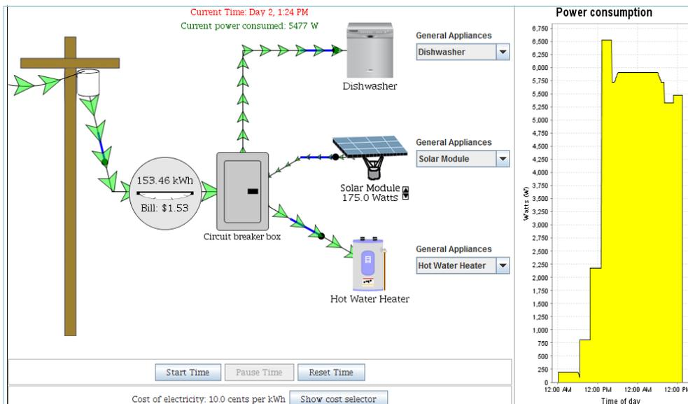
The applet shows power flowing through the transformer drum, the kilowatt-hour meter and into the circuit breaker panel. From the panel it powers various appliances including video game consoles, kitchen appliances, and light bulbs.
