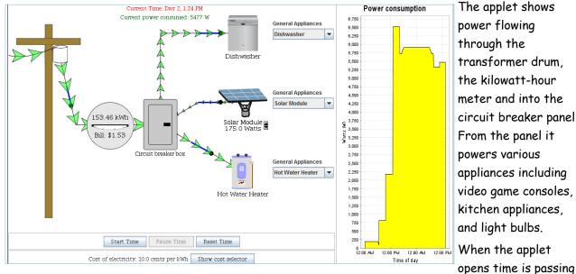
The applet shows power flowing through the transformer drum, the kilowatt-hour meter and into the circuit breaker panel. From the panel it powers various appliances including video game consoles, kitchen appliances, and light bulbs. When the applet
